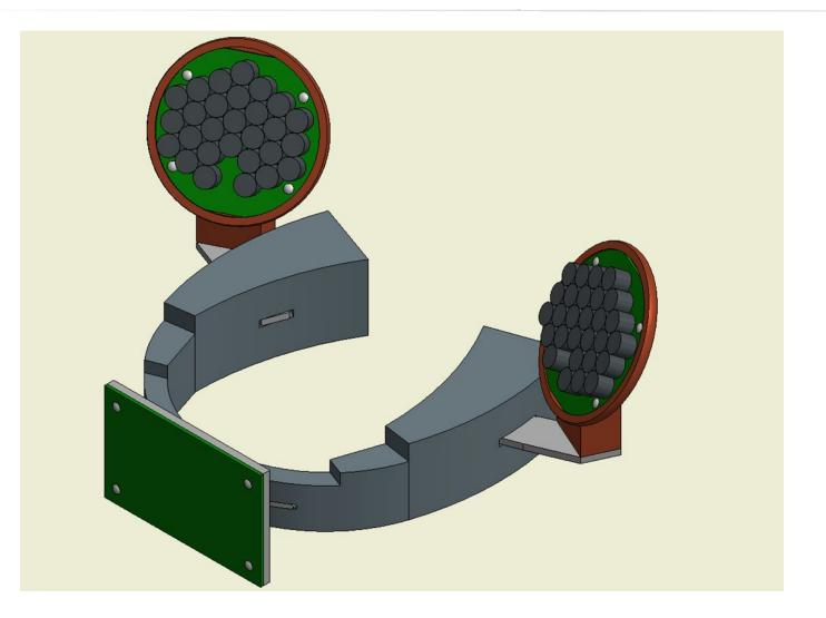
The Collarphone is meant to be worn around the neck, projecting sound from two parametric speaker arrays on both sides of the Collarphone.
